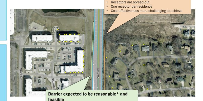
IDOT guidance is to model one receptor per balcony
